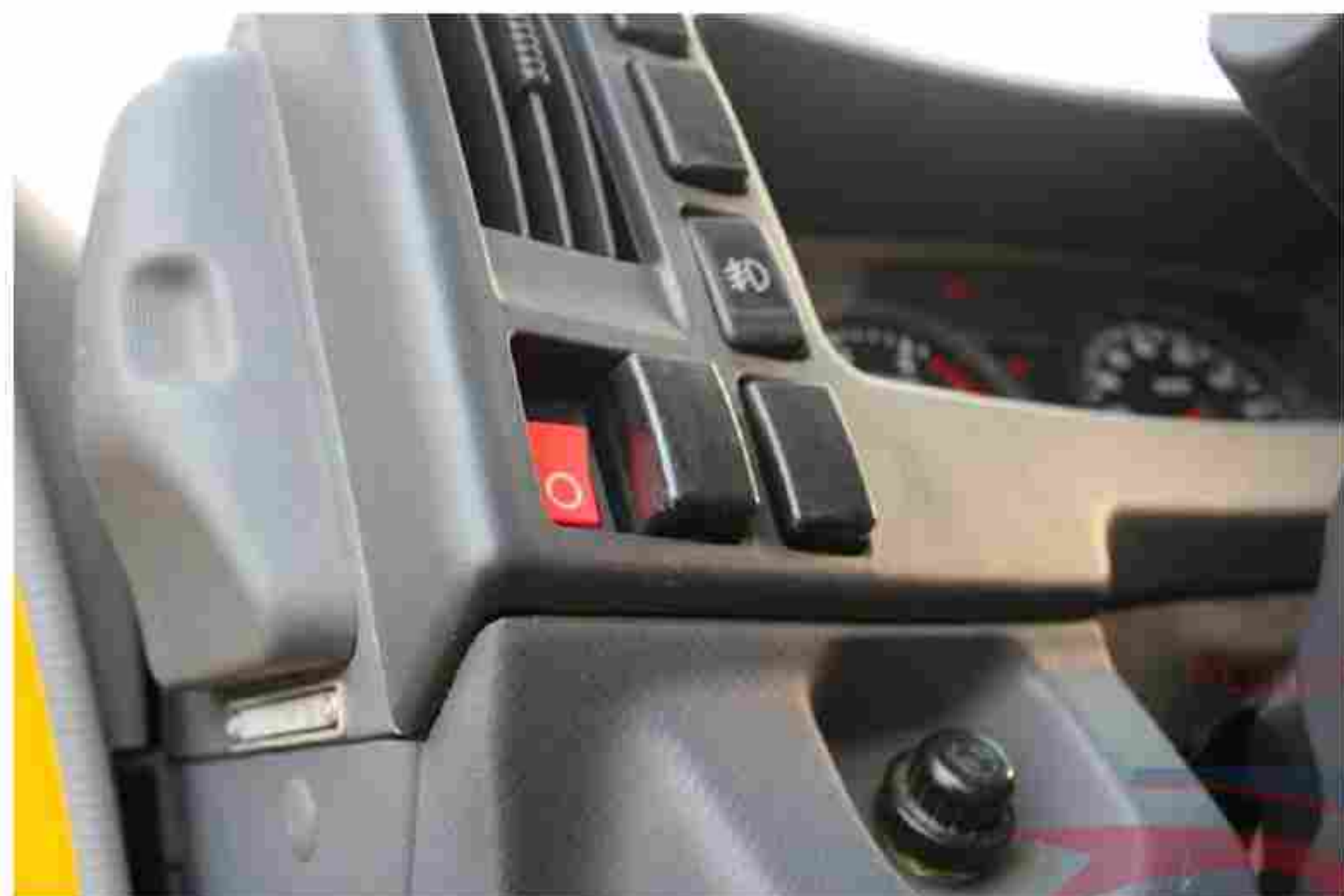
The button in cab can make the light on rear Hydraulic Leg to WORK
