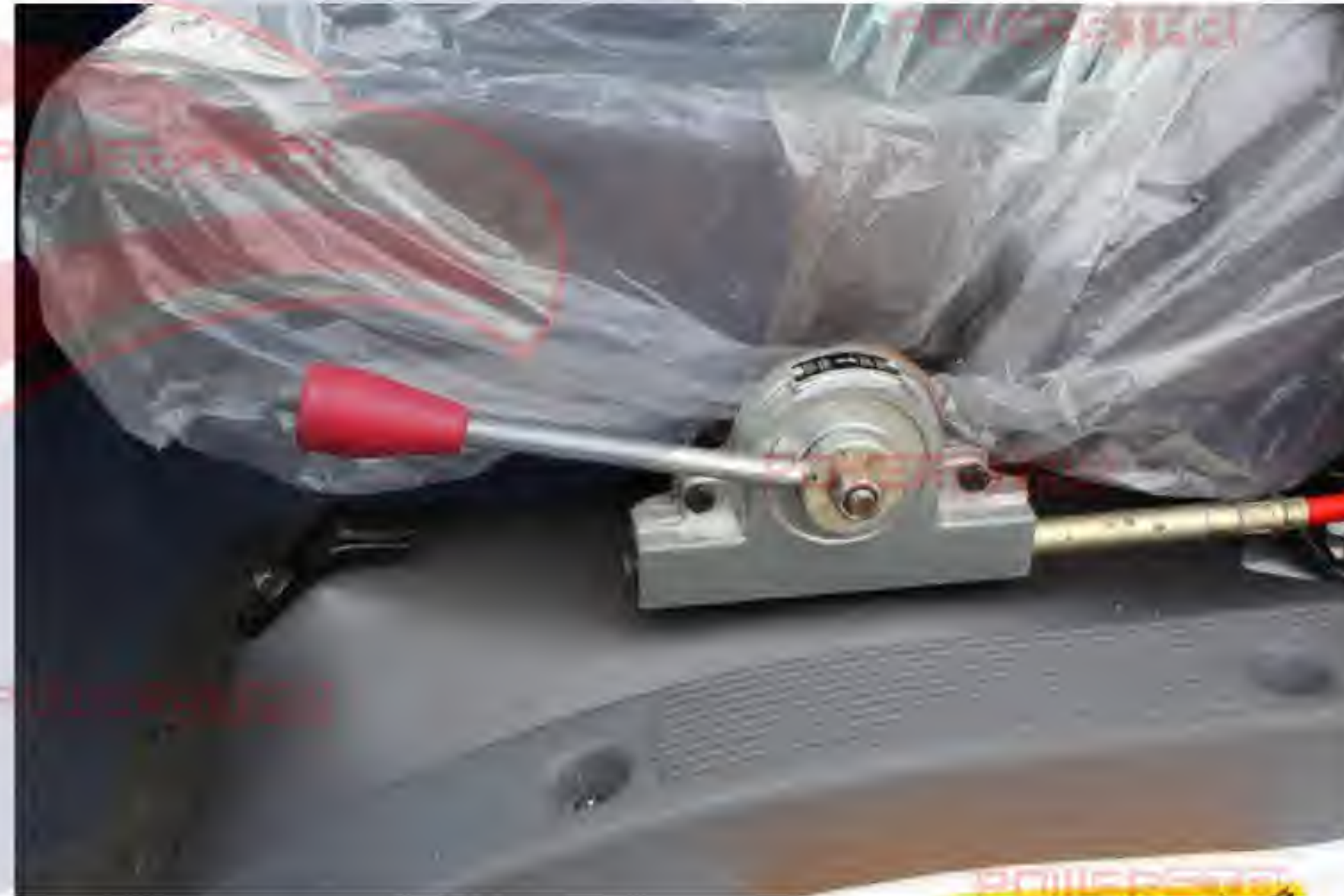
The Joystick at LOWER place The Man Lifter cannot work .
